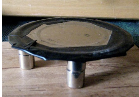
lid of food can with edges taped and Ne magnets underneath
